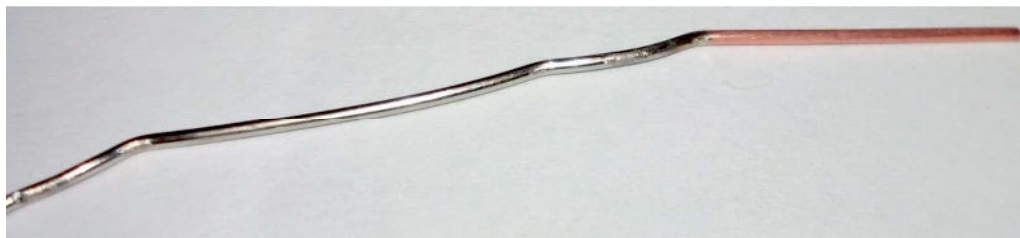
Figure 4.4: steel paper clip covered with copper at the right part
